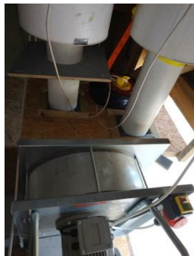
3.13. att. Ozona ģeneratoru kopskats, caurules ozona padevei ventilatoram.
