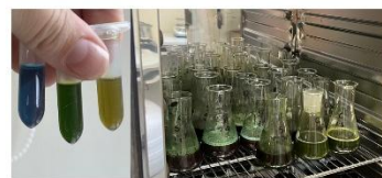
Figure 7. Color variation of extracts under different extraction conditions and experiment setup with heating at 70 °C.
